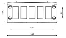
The DES 24 CLICK splittable frame allows to accomodate up to 40 cables with or without connectors with diameters from 2 to 32 mm.
