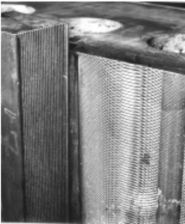
Example for roughening of the surface to be coated by planing (lh.) and milling (rh.)
