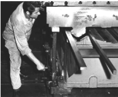
ill. 13: V-guides of the table of a milling machine For the separation of the counter guiding of big components additional means are used (e. g. a winch) to relieve the crane.
