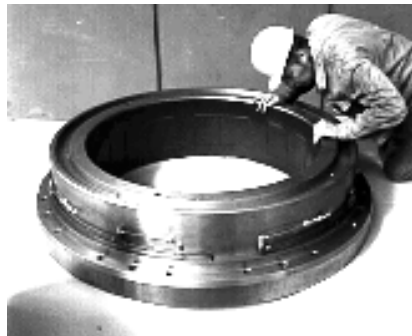
ill. 11: Hydrostatic bearing ring of a crank-stroke milling machine with moulded pockets
